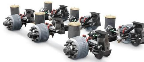
The wheels that enable the trailer to move, the braking system that provides stopping, and the mechanical or pneumatic suspension system that provides driving comfort are considered as sub-components which form the axle units.
