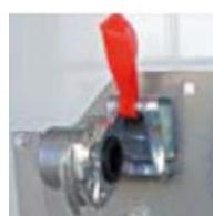
Suspend brake hoses after disconnection. Thus, it prevents possible sand / pollution that can enter the EBS modulator by means of compressed air lines.
